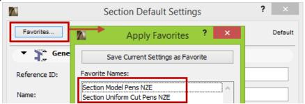
The Section Model Pens NZE uses the Fills & Pens as per the settings in all of the elements the Section cuts through while the Section Uniform Cut Pens NZE Favorite uses the same pen for all Cut elements. Regardless of which Favorite you choose New Viewpoint will be created in the Project Map and the Marker will reference the Drawing on the Layout of the Section when you document it and, of course, uses the Doc: Sections layer.
